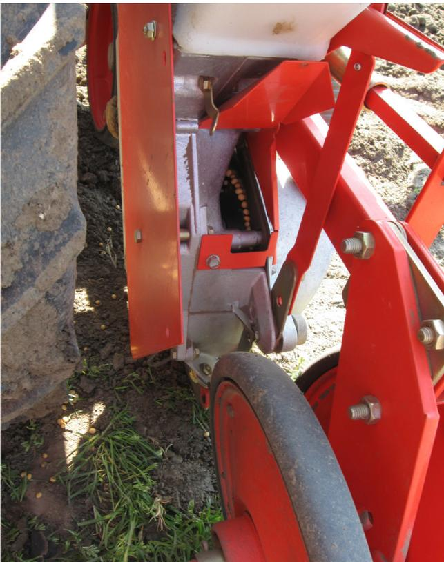
Seeding mechanism in pneumatic precision seeding machine. Photograph: IFVCNS
