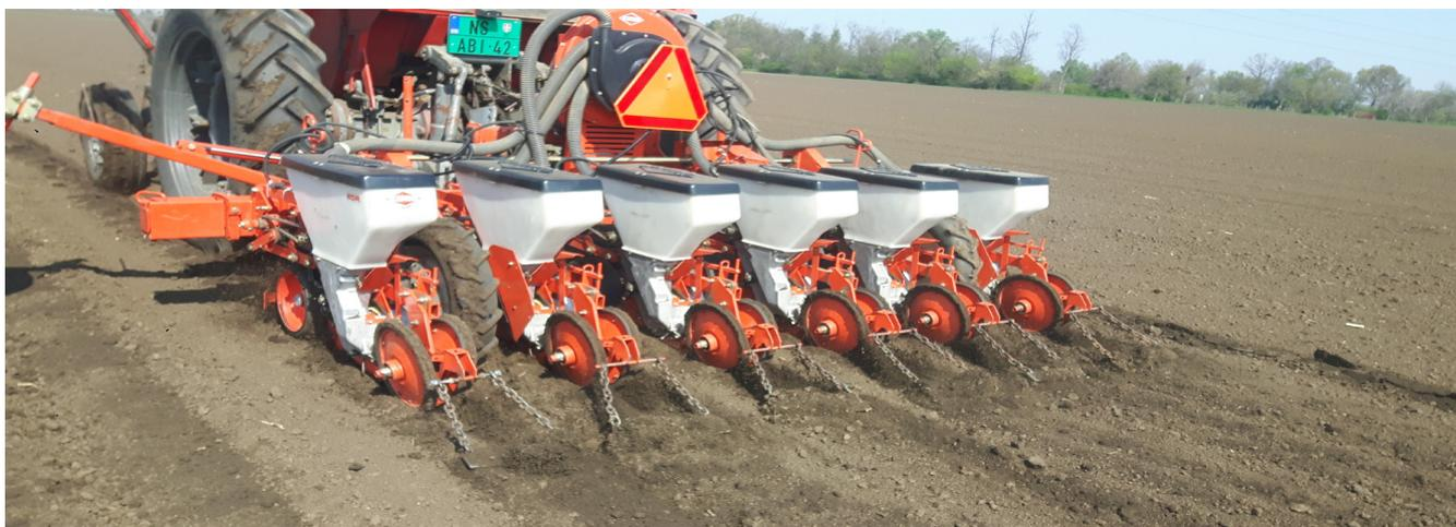
Pneumatic precision seeding machine for soybean. Photograph: IFVCNS
