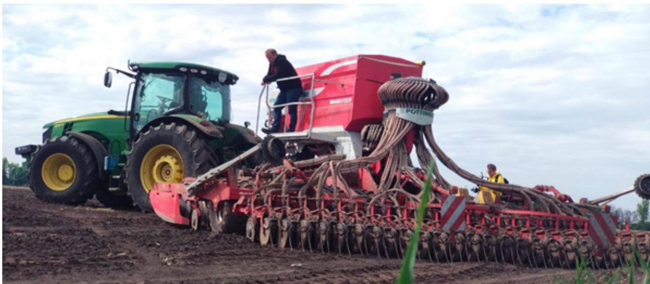
Grain sowing complex Pöttinger, with pneumatic seed metering/delivering mechanism, provides row width of 125/167 mm, or 250 mm. Photograph: Mykola Bykov (Donau Soja Ukraine)
