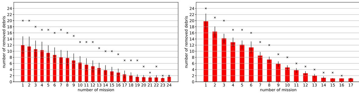
**FIGURE 6.** Number of debris removed per mission in 1000 different runs of (left) incremental greedy search and (right) incremental BS with  $bw = 30$ . The black crosses mark the biggest positive outliers, i.e. a trajectory that would be most likely part of the final solution.
