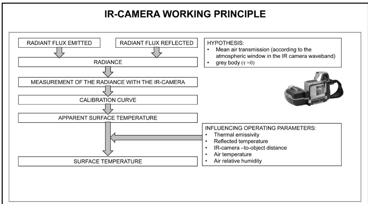
Figure 2. IR-camera working principle.
