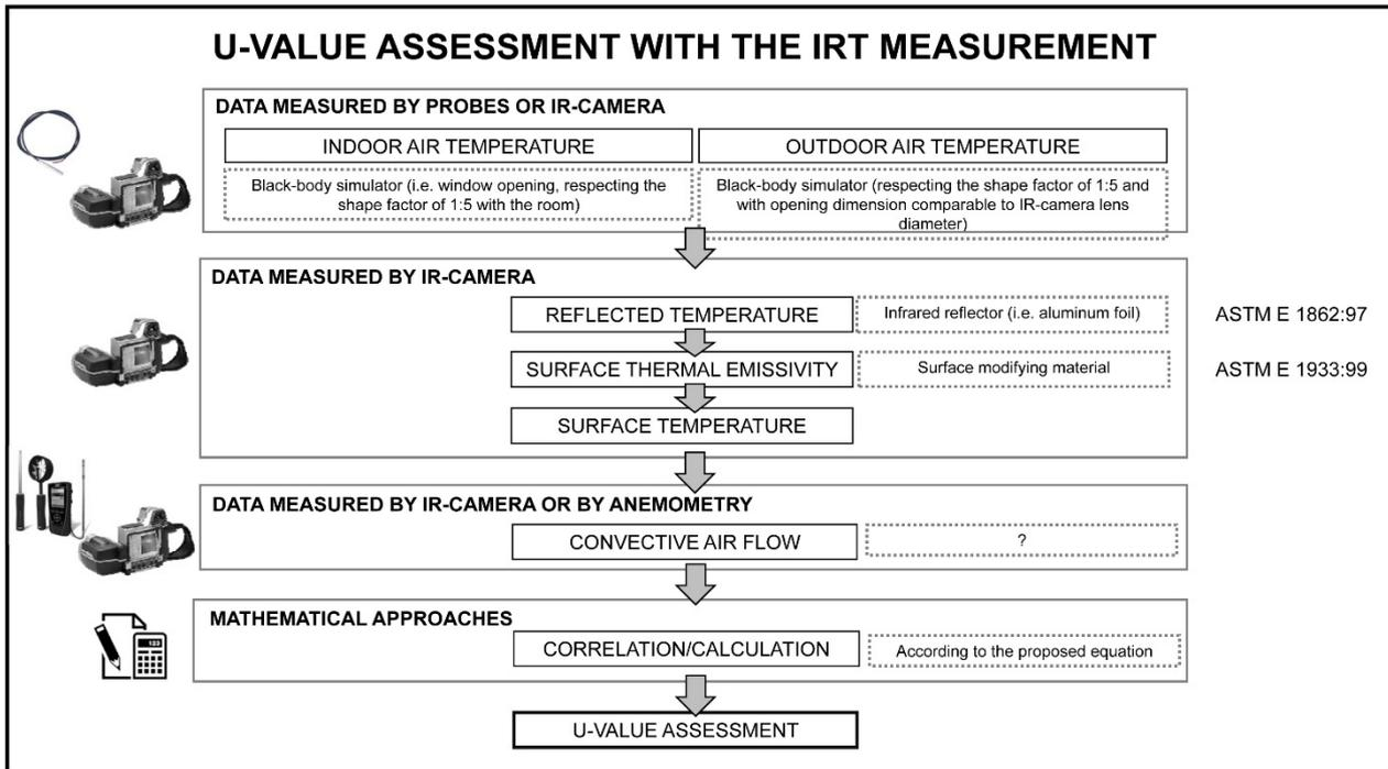
Figure 6. U-value assessment with the IRT measurement.
