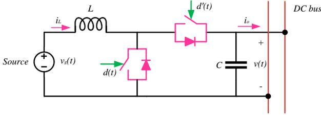
Fig. 4 Circuit of interface converter—bidirectional Boost type.
