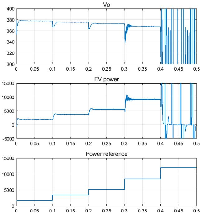
Fig. 9 Oscillation occurs when the EV charging power stepping.
