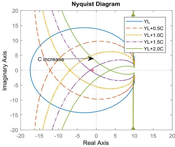
Fig. 6 Nyquist diagram of terminal admittance of double loop control.
