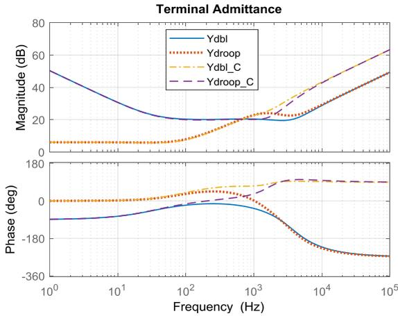
Fig. 7 Terminal admittance shaping by droop control.
