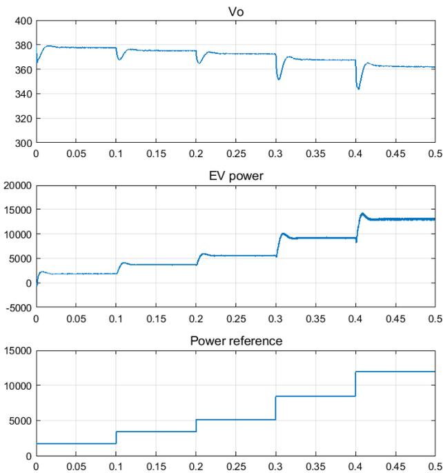
Fig. 10 Terminal capacitor compensation to stabilize the system.
