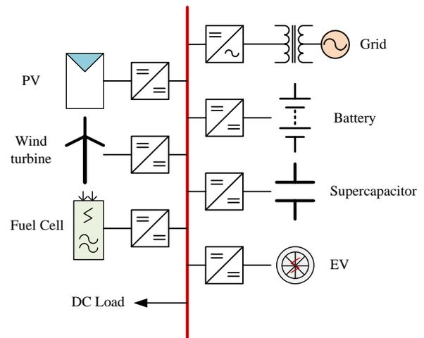
Fig. 1 DC microgrids configurations
