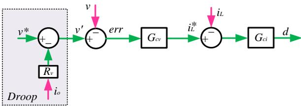
Fig. 5 Control blocks with droop control for interface converter.
