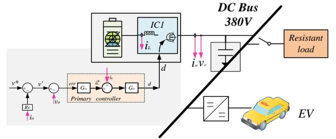
Fig. 8 System model confirmation in simulation.
