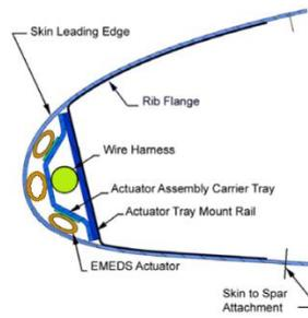
Figure 5 Electro-Mechanical Expulsion Deicing System [1]
