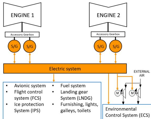
Figure 4 Onboard system scheme
