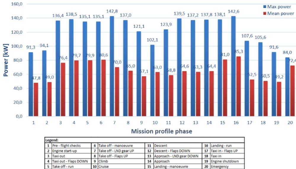
Figure 7 Mechanical power offtake
