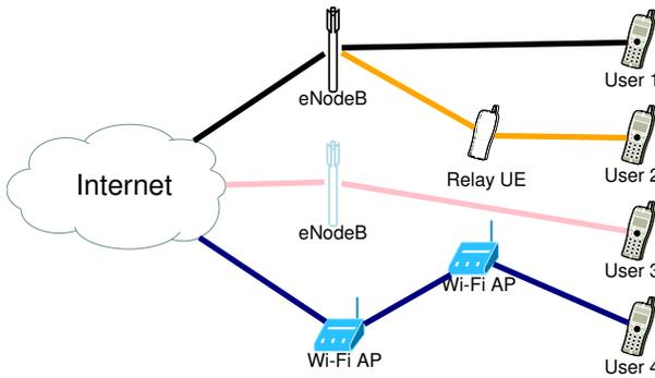
Figure 4: Example graph. Users 1–4 connect to the Internet through a cell belonging to their operator, roaming, D2D, and Wi-Fi respectively.
