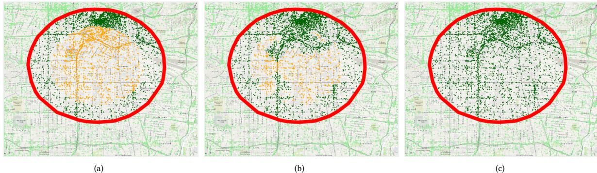
Figure 8: Los Angeles, scenario when the disaster area (enclosed by the red line) is 30% of the total topology. Location of unaffected (pale green), reconnected (dark green), isolated (orange) users, under the roaming (a), D2D (b), AHD (c) remedy strategies.
