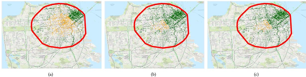
Figure 7: San Francisco, scenario when the disaster area (enclosed by the red line) is 30% of the total topology. Location of unaffected (pale green), reconnected (dark green), isolated (orange) users, under the roaming (a), D2D (b), AHD (c) remedy strategies.
