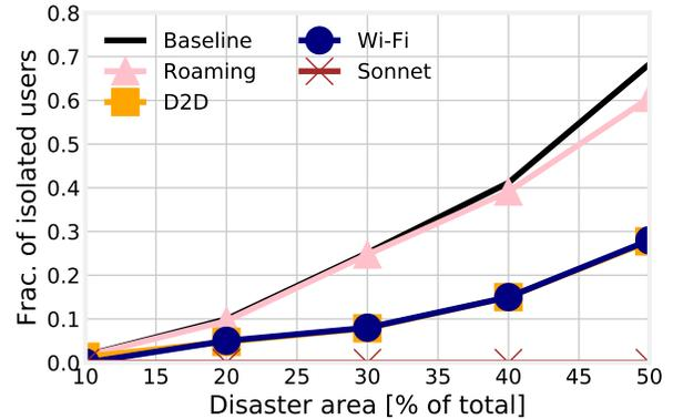
Figure 6: Los Angeles trace: fraction of isolated users as a function of the disaster area size, for different sets of remedy strategies. Remedy strategies are applied in cascade, in increasing order of complexity, e.g., the “D2D” line refers to the case when both roaming and D2D are enabled.
