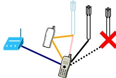
**Figure 1: Connectivity options of a mobile user whose cell has become unavailable due to a disaster (dotted black line), in counter-clockwise order: connecting to a different cell of the same operator (black line); connecting to a cell of a different operator (blue line); use a device-to-device link to reach the Internet (orange lines); using a Wi-Fi access point (pink line).**
