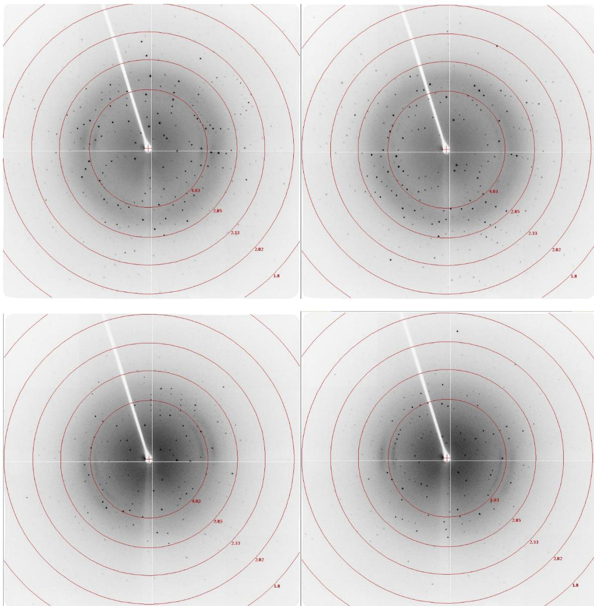
**Figure 4.** Diffraction images with USP5 Zf-UBD crystals in 1.8 M ammonium sulfate, 0.1 M sodium cacodylate pH 5.5, 0.2 M sodium acetate, 1.7 mM L-glutathione reduced, L-glutathione oxidized
