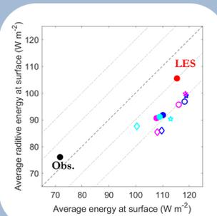
Observed surface energy (black) during hour 12 – 48, is less than the LES (red). Both have smaller contributions from the turbulence fluxes than the SCM/AOSCM but with opposite sign.
