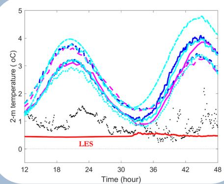
The observations (black dots) are taken at about 25 m above surface. The diurnal variation in 2-m temperature in the model comes from the skin temperature that is allowed to change even though the ice is melting.
