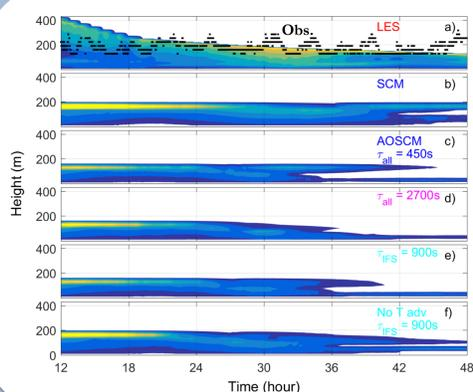
The evolution of the cloud differs between model configuration. Black dots show observed cloud top height.
