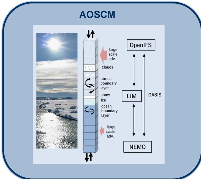
**WHY?** An Atmosphere Ocean Single Column Model (AOSCM) is developed to be used as a tool for model development and process understanding when the coupling between the atmosphere and the ocean is of great importance. This is particularly the case for the atmosphere over the sea-ice covered Arctic Ocean.
