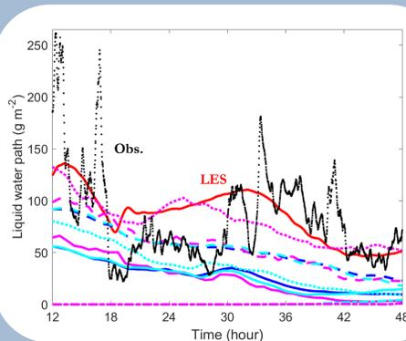
The observations (black) show large temporal variability. The LES has more cloud liquid water than the SCM that has more than the AOSCM. An almost constant difference between the SCM and the AOSCM is detected.
