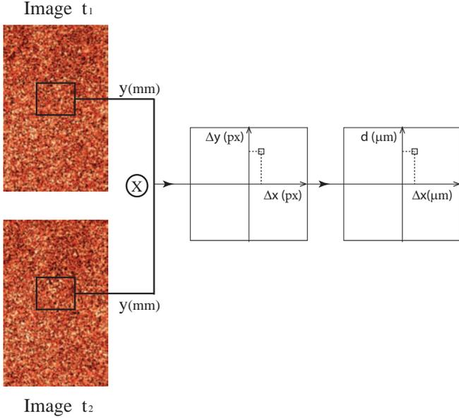
**Fig. 3.** Schematic representation of the imaging set-up in PIV. The position of the cross-correlation peak gives the displacement.
