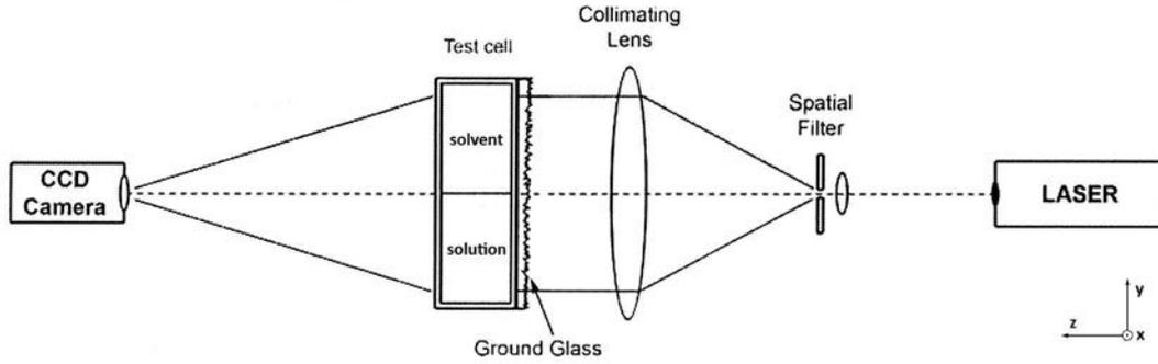
Fig. 2. Experimental set-up for diffusivity measurements by Digital Speckle Photography
