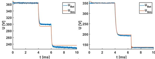
Fig. 7. Simulation and experimental results for the Battery converter's output voltage with a droop constant of 26 W/V (left) and 13 W/V (right)
