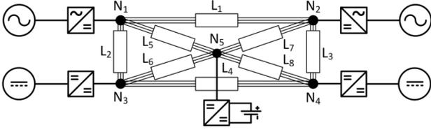
Fig. 1. Example of a dc distribution grid (subsection) containing sources, loads and storage
