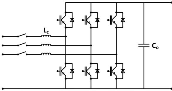
Fig. 5. Topology of the converters that are used in the experimental set-up
