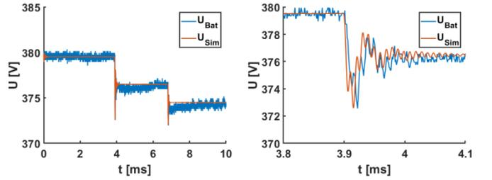
Fig. 8. Simulation and experimental results for the Battery converter's output voltage with a droop constant of 790 W/V
