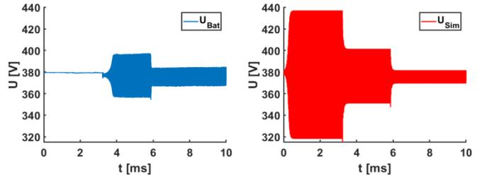
Fig. 9. Simulation and experimental results for the Battery converter's output voltage with a droop constant of 1050 W/V
