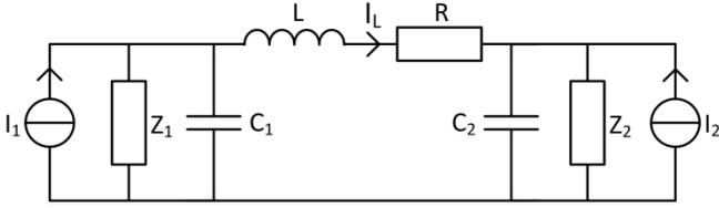
Fig. 3. Simple dc distribution grid with a constant power load (CPL) and a droop source connected via a distribution line.
