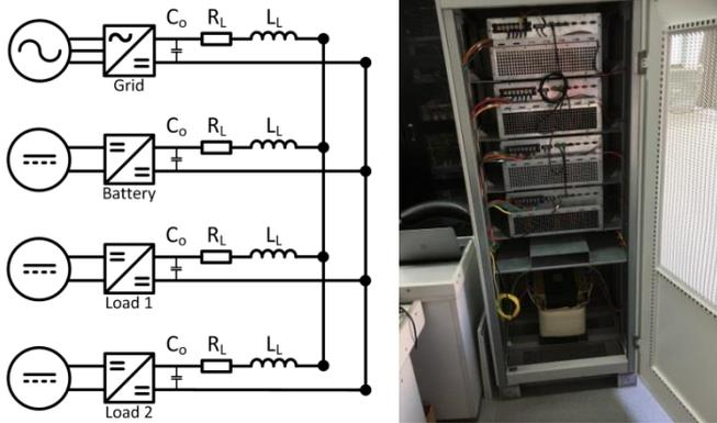
Fig. 4. Schematic (left) and photograph (right) of the DC microgrid set-up consisting of four power electronic converters connected to a dc bus
