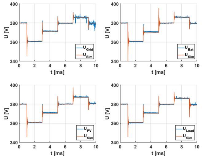
Fig. 6. Simulation and experimental results for the verification of the converter and dc distribution system models
