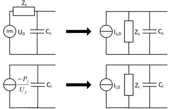
Fig. 2. Ideal and linearized Norton equivalent circuits for droop sources (top) and constant power loads (bottom)
