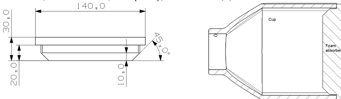
**FIGURE 2.** Foam geometry side view (left) with 30 mm total thickness and 10 x 10 mm frustum (D) – Cup and foam cross sectional view (right)
