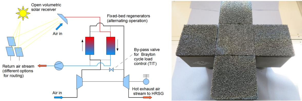
**FIGURE 1.** CAPTURE air-air regenerative heat exchanger concept (left); The ceramic foam absorbers (right)
