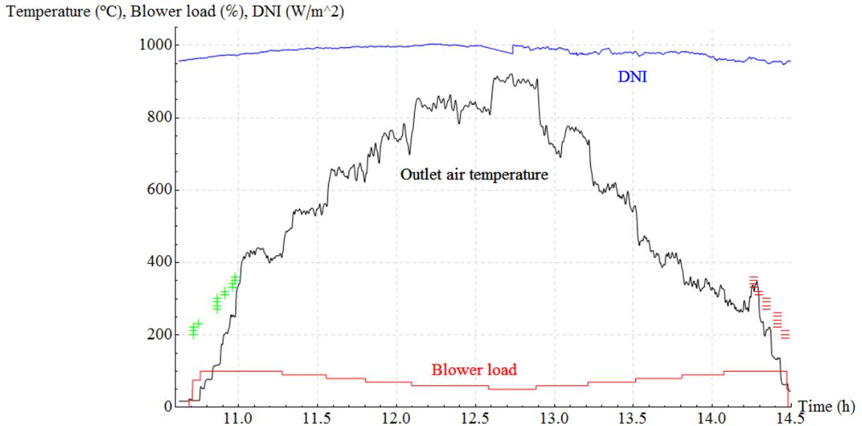
**FIGURE 7.** Experiment performed on the 9th of March 2018 – Receiver outlet air temperature (black), blower load (red) and DNI (blue); heliostat focused (+), heliostat defocused (-)
