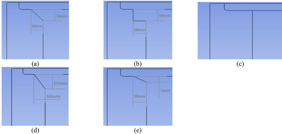
**FIGURE 8.** Foam rear geometries analyzed: (a) 10 x 10 frustum, (b) 10 x 10 square, (c) flat foam, (d) 15 x 10 frustum, (e) 5 x 10 frustum
