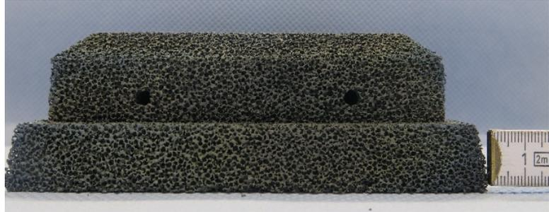
**FIGURE 3.** 3-D view of 2 x 2 cup array to be installed at the tower (left); Ceramic foam absorber side view (right)
