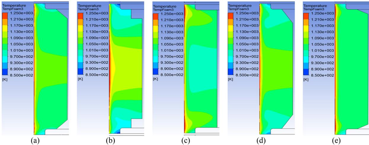
**FIGURE 9.** Contour plots of foam absorber solid phase (ceramic material) temperature
