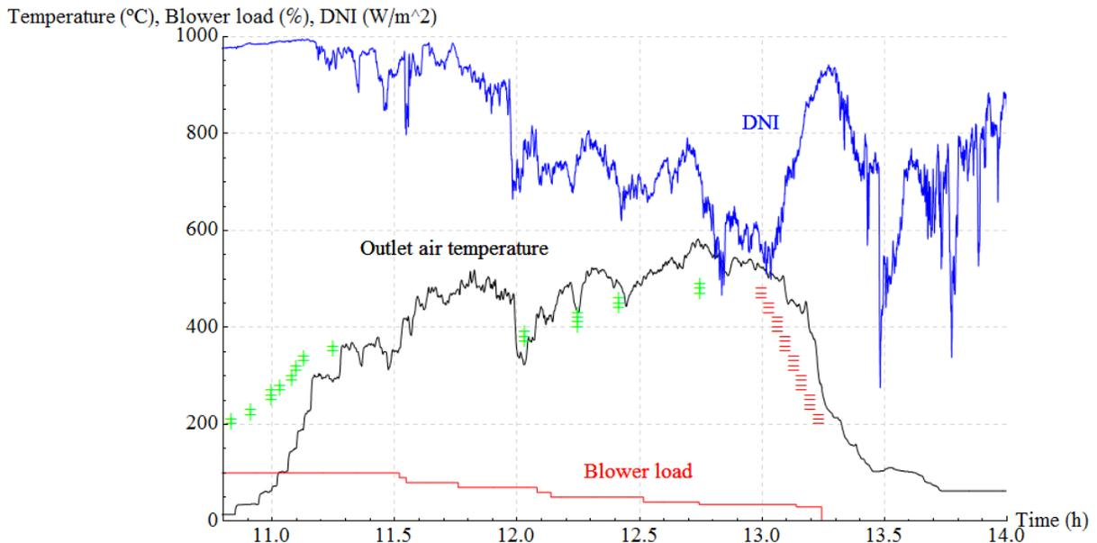
**FIGURE 6.** Experiment performed on the 7th of March 2018 – Receiver outlet air temperature (black), blower load (red) and DNI (blue); heliostat focused (+), heliostat defocused (-)
