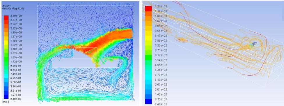
Figure 12: Computational velocity vector field over the piece for a transversal plane located at the  $H_2$  injection area (left). Path lines coming from the  $H_2$  injection (right), colored by temperature.
