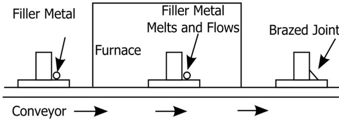
Figure 1: Simplified diagram of the brazing process.
