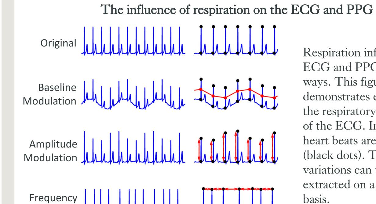
Respiration influences the ECG and PPG in three ways. This figure demonstrates extraction of the respiratory modulations of the ECG. Individual heart beats are detected (black dots). The three variations can then be extracted on a beat-by-beat basis.
