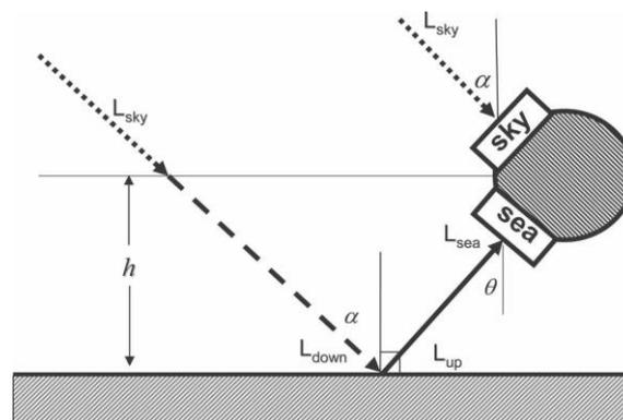
Figure 4: Geometrical set up of the ISAR on RV Investigator (Figure taken from Donlon et al., 2008). In this case the nadir viewing angle,  $\vartheta$ , is 25° and the height,  $h$ , above the ocean surface is typically ~19.6 m.
