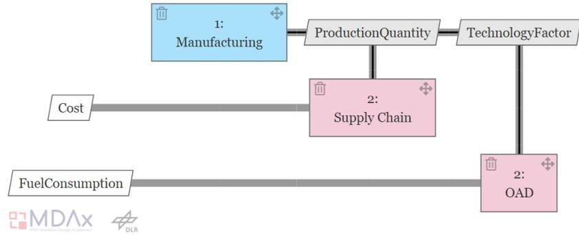
I. XDSM Workflow coupling Mfg Domain and OAD Domain set-up using MDAX
