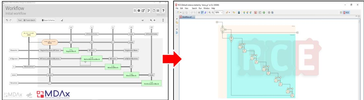
**Figure 7 – Disciplinary tools can exchange information using CPACS as common language [27]; the MDAO process coupling disciplinary competences is then automatically generated using MDAX [28]; the workflow is finally exported and executed in the PIDO RCE [29].**
