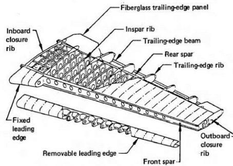
**Figure 8 – Horizontal tail plane structure breakdown [31]**
