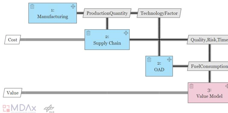
I. XDSM Workflow coupling Mfg Domain, SC Domain and OAD Domain, set-up using MDAX
