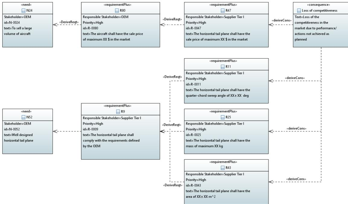
**Figure 10 – OEM’ needs and requirements concerning the supply chain domain (N24) and the manufacturing and design domains (N52) modelled using the new AGILE4Profile, [32]**
