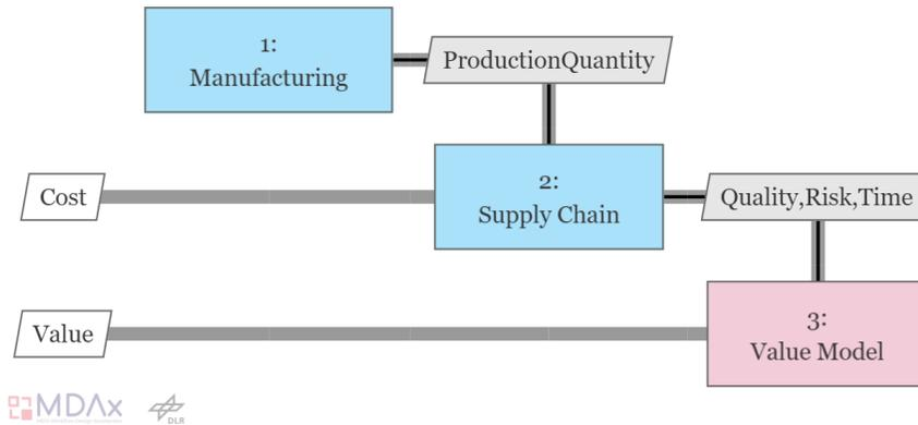
I. XDSM Workflow coupling MfG Domain and SC Domain, set-up using MDax
