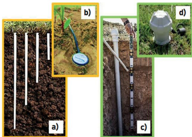
Soil sensors Drill and Drop (a,b) Enviroscan (c,d). Photograph: Gaia Sense
