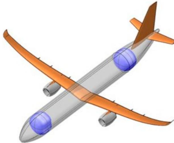
Figure 3: Long-haul aircraft concept proposed by Bauhaus Luftfahrt using LH2 stored in cylindrical fuselage tanks and used for combustion in H2 turbofan engines [3]. Picture adopted from a Bauhaus Luftfahrt source.
