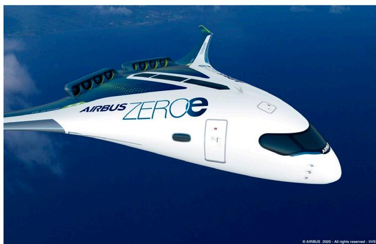
Figure 4: Airbus is investigating the design of BWB aircraft configuration for medium range of 3700km and 200PAX [10]. "Picture adopted from an Airbus source.
