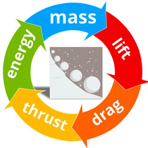
*Figure 7: The snowball effect for aircraft design: Additional mass leads to iterative increases in lift, drag, thrust, energy, and the required mass for airframe and engine systems and structures to account for those increases.*
