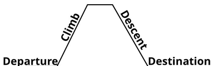
Figure 6: Illustration of a basic flight mission, which essentially includes departure and climb to a certain altitude, and descent to the target destination. Of course, usually a mission also includes cruise flight between climb and descent to travel the intended distance.
