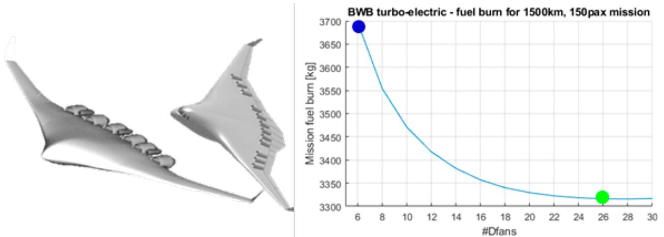
Figure 20: Illustration of the results of the case study 3: For the BWB aircraft, the optimum number of DFs that was found is 26, i.e. with total fan area of  $26\text{m}^2$ . With the 26 DFs, the fuel burn for the 1500km mission is about 3316kg (green dot in the graph). This translates in about 10% reduction in mission fuel burn compared to the initial BWB with 6 DFs which has about 3696kg fuel burn for the same mission (green dot in the graph).
