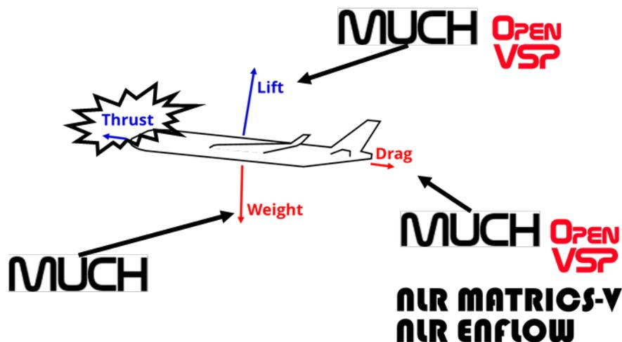
Figure 8: Illustration of various tools in use at NLR in different modelling fidelities for conceptual sizing, preliminary weight estimation and aerodynamic characterization.
