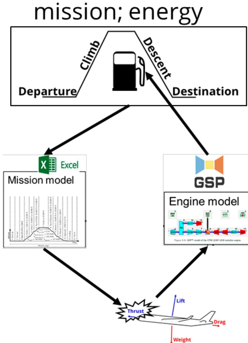
Figure 11: Illustration of the mission fuel consumption, which can be calculated by the accumulation of fuel flow, as predicted here by the GSP engine model, along the whole mission.
