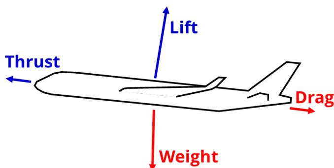
Figure 5: Illustration of the basic force equilibrium in powered flight, where the aircraft depicted is flying at a small climb angle.
