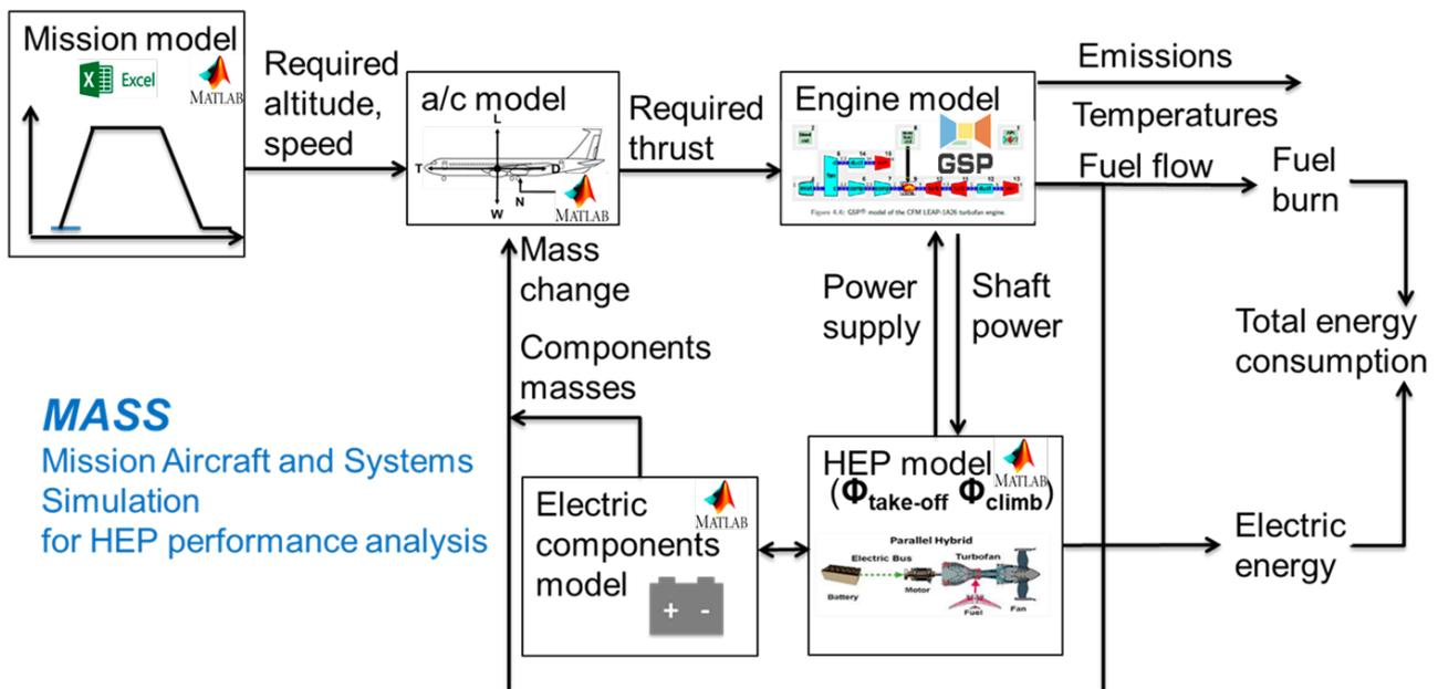
Figure 13: Illustration of the NLR MASS tool [13], which is primarily an integration framework, in which the main required component models can be incorporated from various sources. Note that non-propulsive power demand is not explicitly included in this illustration but of course can be incorporated in MASS analyses.
