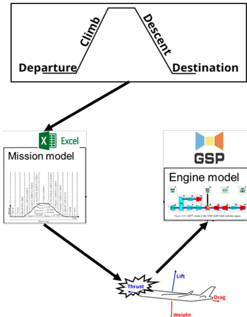
Figure 10: Illustration of the integration of the power required for the thrust force along the flightpath, at the prescribed air speed, which yields the required power supply and energy that is needed for the mission. The required fuel mass flow for a certain thrust requirement, at a given speed and altitude, can be calculated for example with NLR's GSP engine modelling tool.
