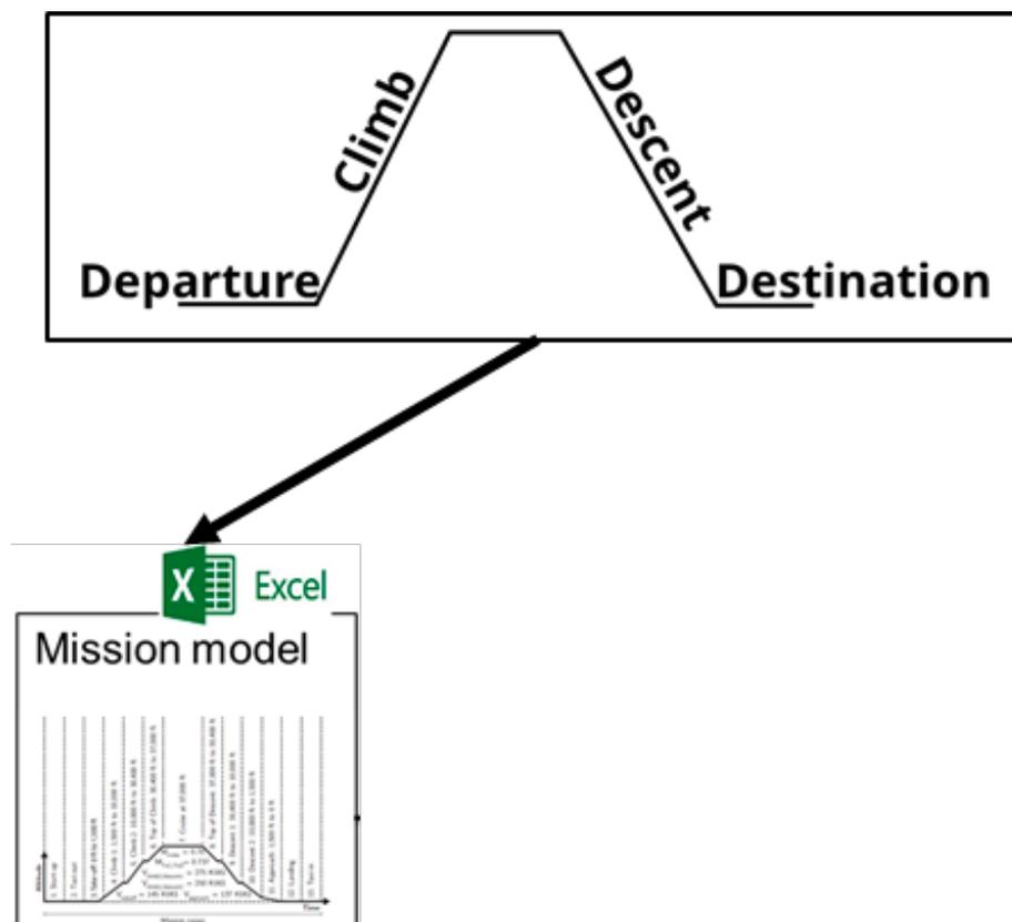
Figure 9: Illustration of the mission representation of the intended flight, which shall define speed and altitude as function of horizontal position for the whole flight including taxi, take-off (TO) landing etc. Activation of devices such as LG, high-lift, ECS, etc. shall also be included. A basic tabular Mission Model is used for this, for example implemented in MS Excel.
