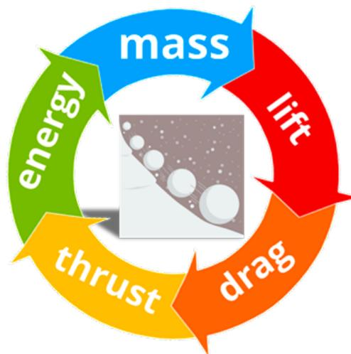
Figure 12: Illustration of the snowball effect in aircraft design: increased mass requires more lift, which induces more drag, demanding more thrust, more energy and more mass, etc.
